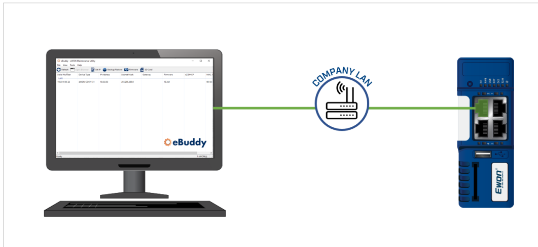
Fig. 26 Connect the computer indirectly to the Ewon though Company LAN
